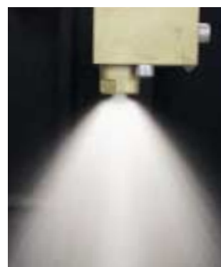
Spray cone at 7 bar water and 2 bar air
